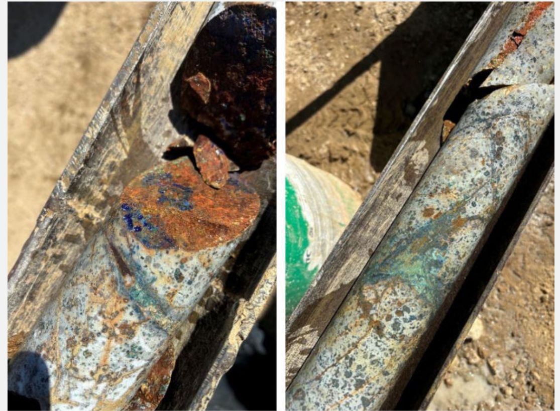
Figure 1: Azurite, malachite, chalcocite in core from MHB-32: 527 to 537 ft (160.6-163.6 m)
